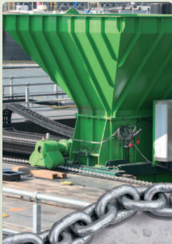
TECDOS Offshore Skidding Systems - Drives for skidways on pontoons above/under ship decks
