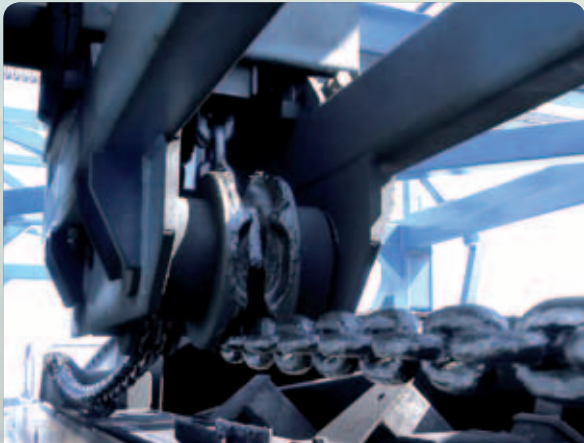
TECDOS Offshore Skidding Systems - Drives for skidways to move ship cranes
