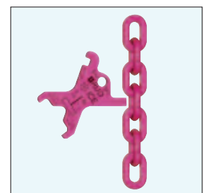
Testing for pitch elongation caused by wear of nominal diameter
