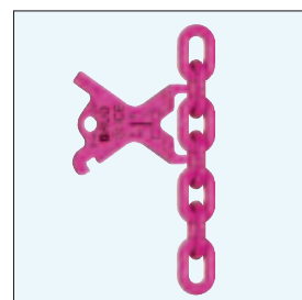
Testing of plastic elongation caused by overload
