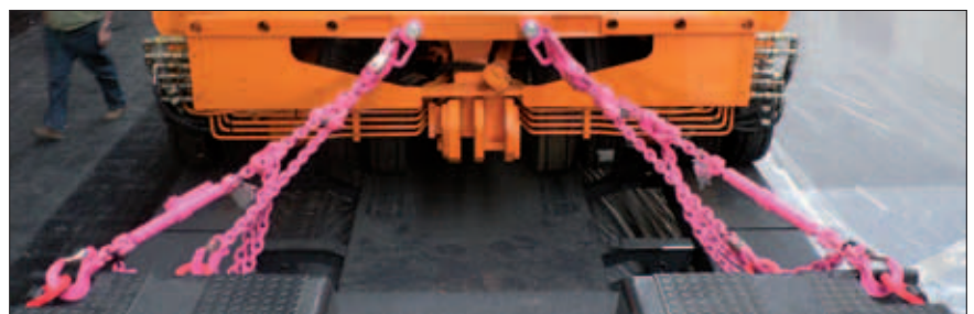
Four bearing strands by VIP lashing chains with special balancer rolls
