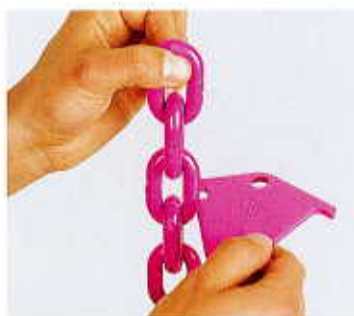
Testing wear of nominal diameter
