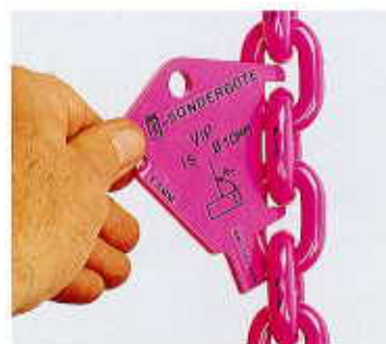
Testing for plastic elongation caused by overload
